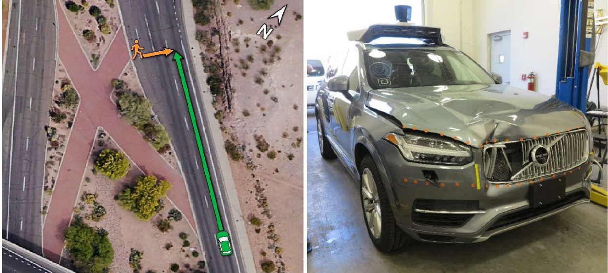
Figure 5 Fatal crash of a Pedestrian and a Highly Automated Vehicle. Left: Path of pedestrian (orange) and vehicle (green). Right: post-crash view of vehicle. Source (NTSA 2018)
