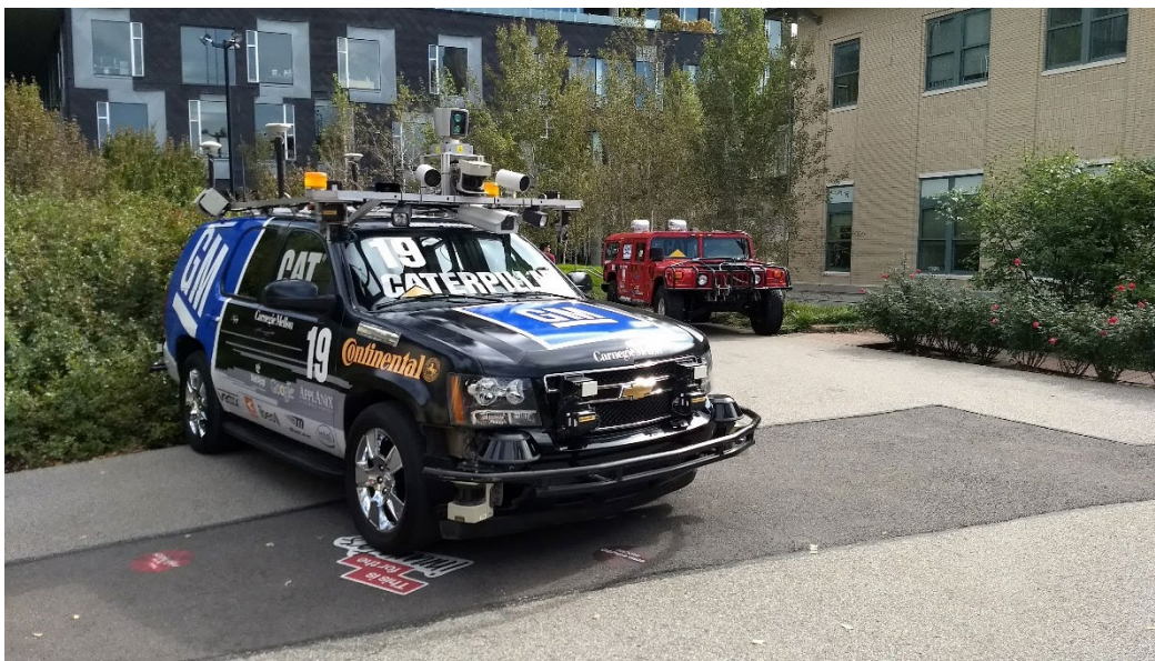
Figure 1: Carnegie Mellon University Automated Vehicle Boss won the 2007 DARPA Urban Grand Challenge and demonstrated the capability of automated vehicles to drive successfully in traffic. Source: Photo by Chris Hendrickson
