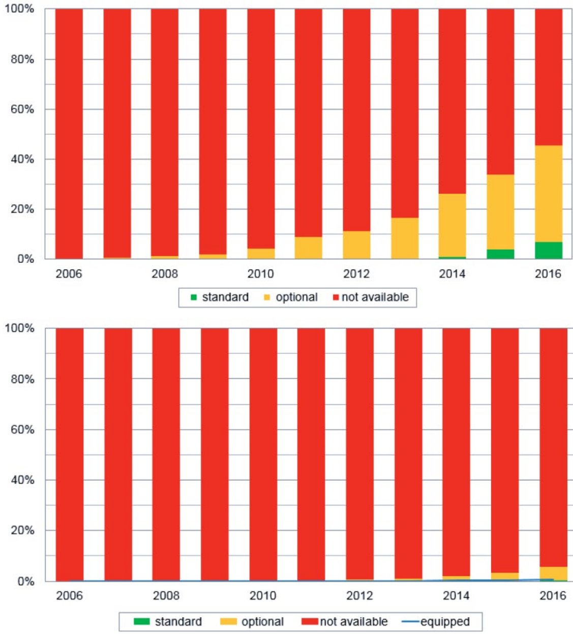
Figure 3 Share of new vehicles offering automatic emergency braking (top) and registered vehicles equipped with the feature (bottom). Source: NASEM 2018.
