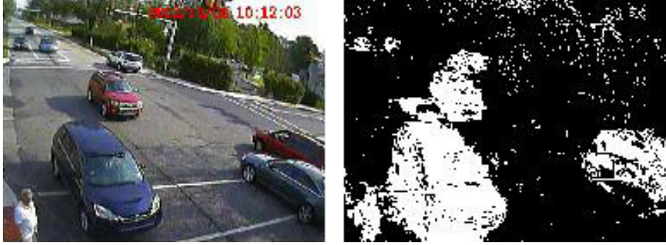
(a) A frame (left) and its binary foreground image (right). Note that the red car’s shadow connects with the blue car in front.
