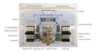
Figure 1: ProtoDrive Platform with coupled vehicle and load motors, battery and super capacitor.
