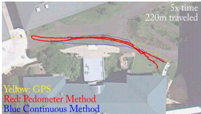
Figure 4: Comparison between implemented dead-reckoning algorithms over a 220m run outdoors at Carnegie Mellon University campus.
