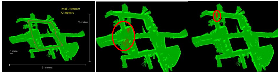
Figure.8: Particle filter estimate over time for environment 2. The standard deviation of the PF bubble is \sim 1\text{m} after convergence over the duration of the run
