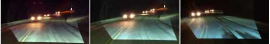
Fig. 6. View shown from the perspective of the vehicle equipped with our prototype. Left: Anti-glare feature is disabled acting as a typical high beam. Middle and Right: Anti-glare feature is enabled detecting multiple oncoming vehicles and reducing light only in the direction of each driver. Notice no discernable difference between images.
