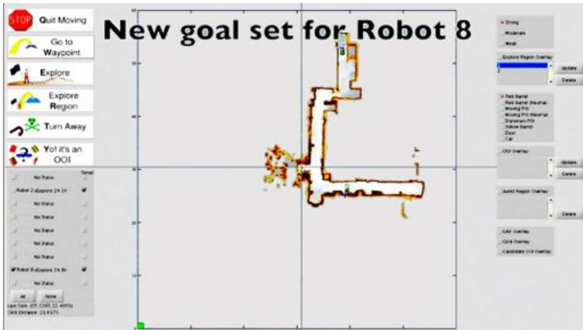
Figure 21: Ground control display of the Strategy/Plan operator with intuitive human-machine interface controls.
