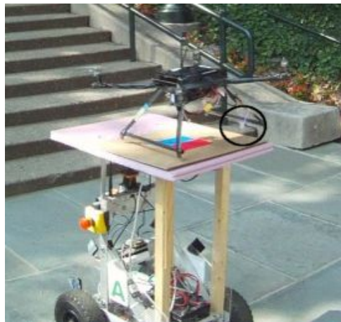
Figure 22: Magnetic tailhook system used to assist aerial quadrotor landing and mating on a ground robot.
