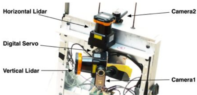
Figure 6: Detailed view of the sensor suite consisting of a panning high resolution camera, omnidirectional camera, horizontal and vertical LIDAR scanners.
